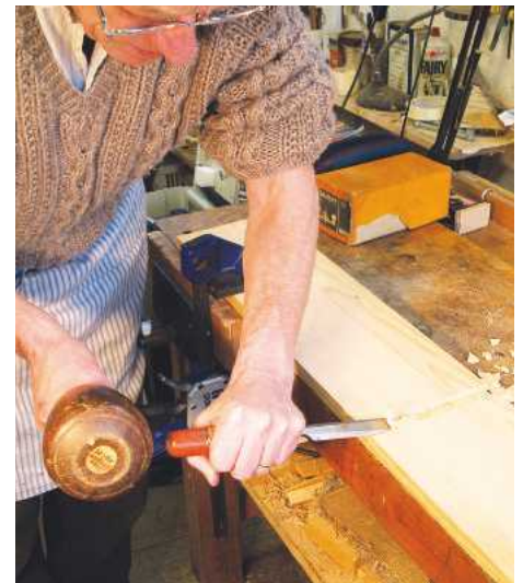
▲ Pic.4 Coming back in from the other side to avoid breakout
